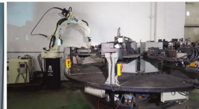
全自动机械手电焊 Full-automatic electrowelding by manipulator
